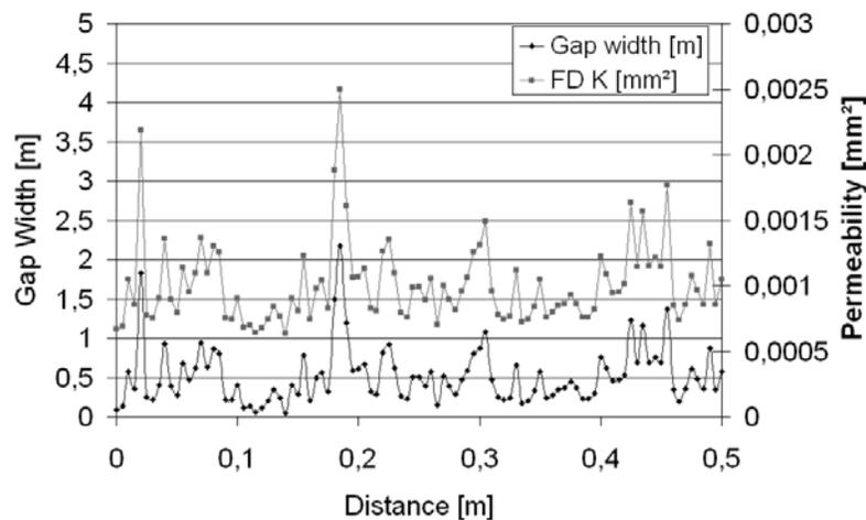
Fig. 2 Correlated gap width and corresponding permeability value.
