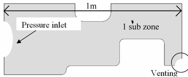
Fig. 4 Model with race tracking.
