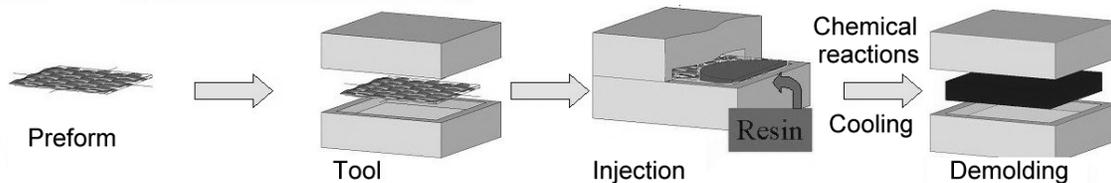
Fig. 1 Schematic showing the different stages of the RTM process.
