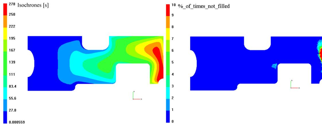
Fig. 5 Filling pattern in case of a deterministic study no air entrapments (left). Possibility to have an air entrapment in case of a geometry sensitive to race tracking (right).
